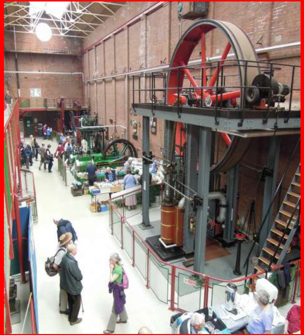
A unique true vertical cross-compound engine, rescued from a mill in Denby Dale
